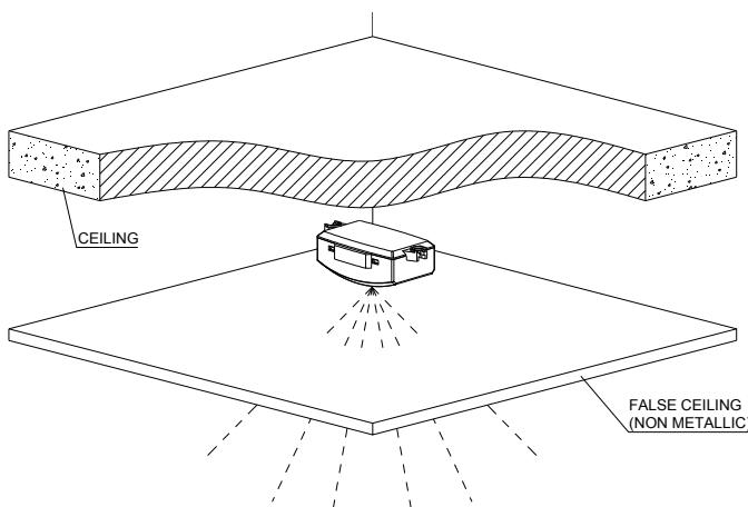
The sensor must be facing to the zone where we want to detect.
