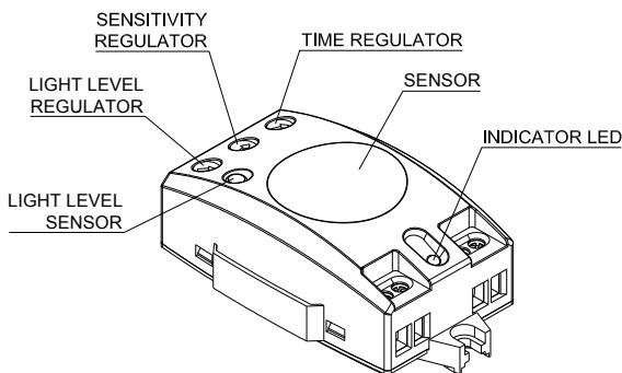
The ECOMAT MINI 2N presence detector is capable of detecting the slightest movement because of its high-frequency technology. Its detection precision does not depend on the ambient temperature. It immediately detects any movement, even those of inert elements, such as doors or chairs.
