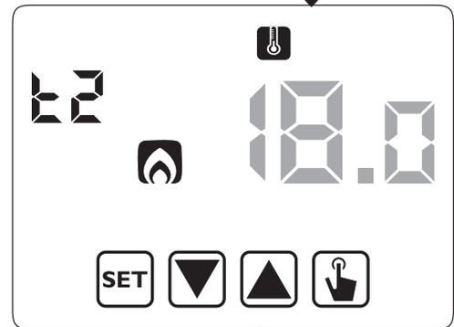
5. The value of the flashing T3 temperature is displayed. Modify the value with the keys ▲ and ▼ and press the key ⏏ to go back to the page of T1 temperature.
