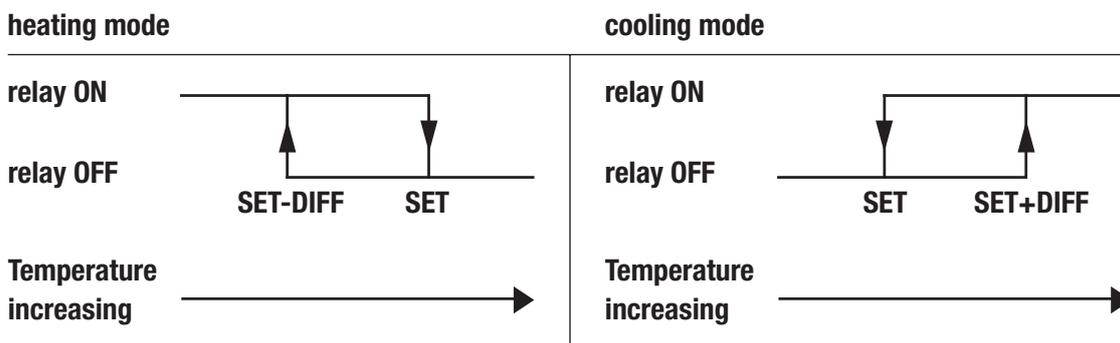
where SET represents the setpoint and DIFF the hysteresis (useful to avoid continuous switches on/switches off dangerous for the system in proximity to the reaching of the setpoint).
