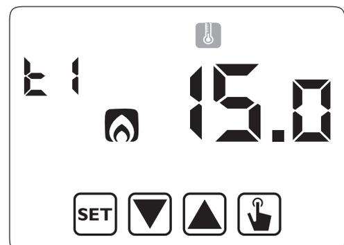
3. The value of the flashing T1 temperature is displayed. Modify the value with the keys ▲ and ▼ and press the key ⏏ to move to the modification of T2.
