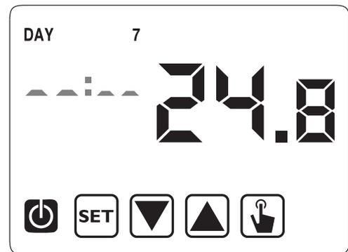
**The programmable thermostat remains in off operation condition until when the hour is not inserted, ensuring in this way the saving of the antifreeze temperature (6°C).**
