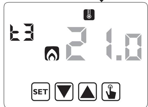
6. Once all parameters are set, to exit and to go back to the programming menu, press for a short time the key SET. To exit and to go back to the normal operation press for a long time the key SET or wait for the time-out expiration (30 seconds about).
