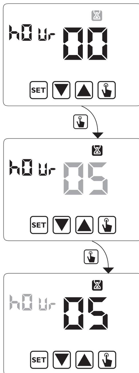
5. Once all parameters are set, to exit and to go back to the programming menu, press for a short time the key
